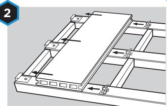
Place the first piece of decking on the subframe with the decking running perpendicular to the joists. The first piece of deck should be secured with starter clips. **Do not screw or nail through** *HD Deck XS® Fire*, use one Slim Clip and screw on every joist.
