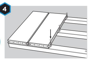
Take the next piece of deck and securely push into the Slim Clips. Now nip the screw to secure the Slim Clip against the board. **Do not over tighten**. Repeat steps 3 and 4 to cover the deck, using one Slim Clip and screw on every joist.
