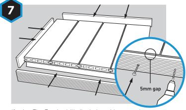
If using Fire Fascia, drill pilot holes with counterbore through the fascia at 200-300mm intervals. According to ambient temperature allow a 5-7mm gap between end of deck board and the fascia. Screw fascia to the joist. Always screw fascia to the joist at a 90° degree angle.
