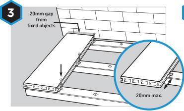
To secure the first board, use one Slim Clip and screw on every joist. Take a screw, place in the hole located in the Slim Clip and screw into the subframe. Make sure the boards do not overhang the joist at the edge by **more than 20mm** and a **20mm expansion gap** should be left between the wall or other fixed objects surrounding the deck.
