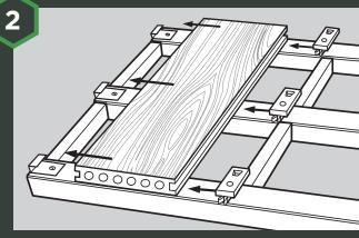
Place the first piece of decking on the timber frame with the decking running perpendicular to the joists. The first piece of deck may be secured with starter clips. **Do not screw or nail through** *HD Deck® Dual*, use one Universal Clip and screw on every joist.
