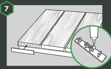
If using end caps, apply a high quality grab adhesive to the end caps to secure for extra adhesion. Wipe away any excess from the edge of the cap.
